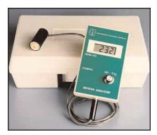
The CON-TROL-CURE® Oxygen Meter Test Kit is indispensable for measuring percentages of oxygen in inert atmosphere curing systems. The sensor measures atmospheric oxygen from 0-100% and is not affected by hydrogen sulfide or carbon dioxide. Maintenance-free, its unique galvanized electrode has an extended life expectancy of 3 to 5 years at a standard temperature of 25°C. Comes complete with the meter and 5-ft electrode, screwdriver, instructions, and carrying case.
