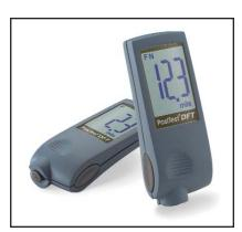
Choose between two models of this basic, electronic gauge. Ferrous for steel or Combo for steel and aluminum. This pocket-size and lightweight gauge features a large LCD, a built-in probe, and simple operation.
