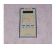
The UV-Power Integrator 06 is a small, only 6 mm flat, self-contained, pass-through UV-Microprocessor Integrator. It is specially designed to measure, record and display peak UV intensity, UV dosage, and optionally (UV-T) temperature, in the UV curing process of narrow web presses and in some applications of the flexo print.
