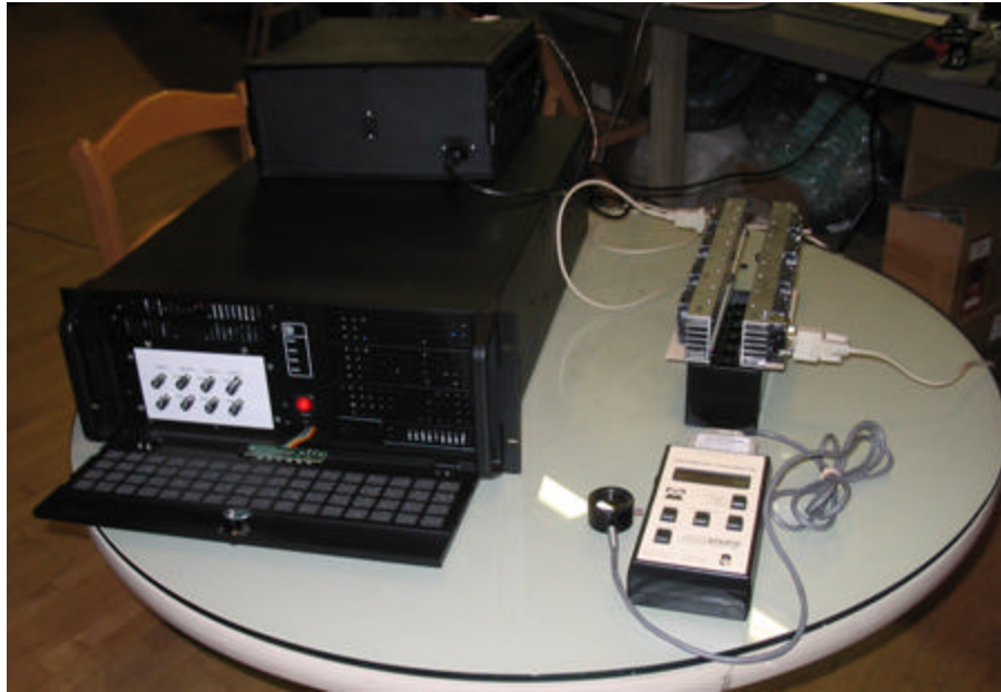
Figure 1 - Power Supply, Lamps on Pallet Fixture and Radiometer
